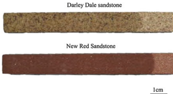
Fig. 3.3 Permeability experiments of Darley Dale sandstone and New Red sandstone
