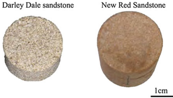
Fig. 3.4 Darley Dale sandstone and New Red sandstone, cut into cylinders for ultrasonic velocity measurements
