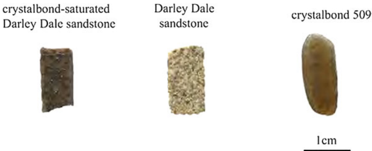
Fig. 3.5 Darley Dale sandstones, prepared with crystalbond 509, for DMA experiments
